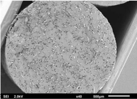
**Fig 5: SEM image of a fracture surface of an extruded 3D printing-wire with 10% Danufile and 90% PLA (PLA 3251D); recording of complete wire cross section; the incorporated fibres exhibit a uniform distribution in wire.**
