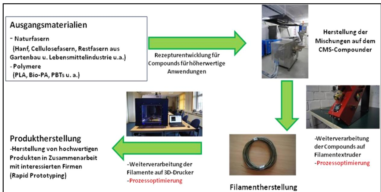
Fig. 2: Process chain for the production of NFK products via 3D printing
